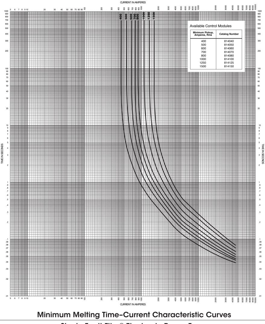
Single Fault Fiter® Electronic Power Fuses Inverse-Curve-Type Control Modules
